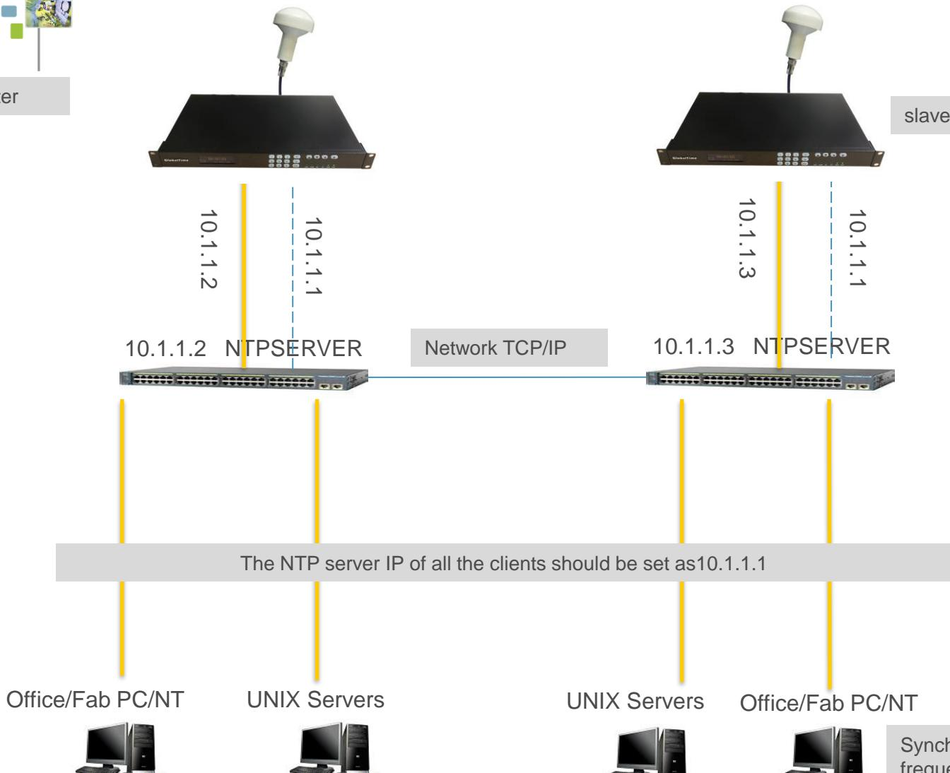
When there are network problems, both the master and slave will use the virtual IP 10.1.1.1. As soon as the network problems are solved, the IP 10.1.1.1 will float to the server whose status is better than the other's, and the other server will not use the virtual IP.
