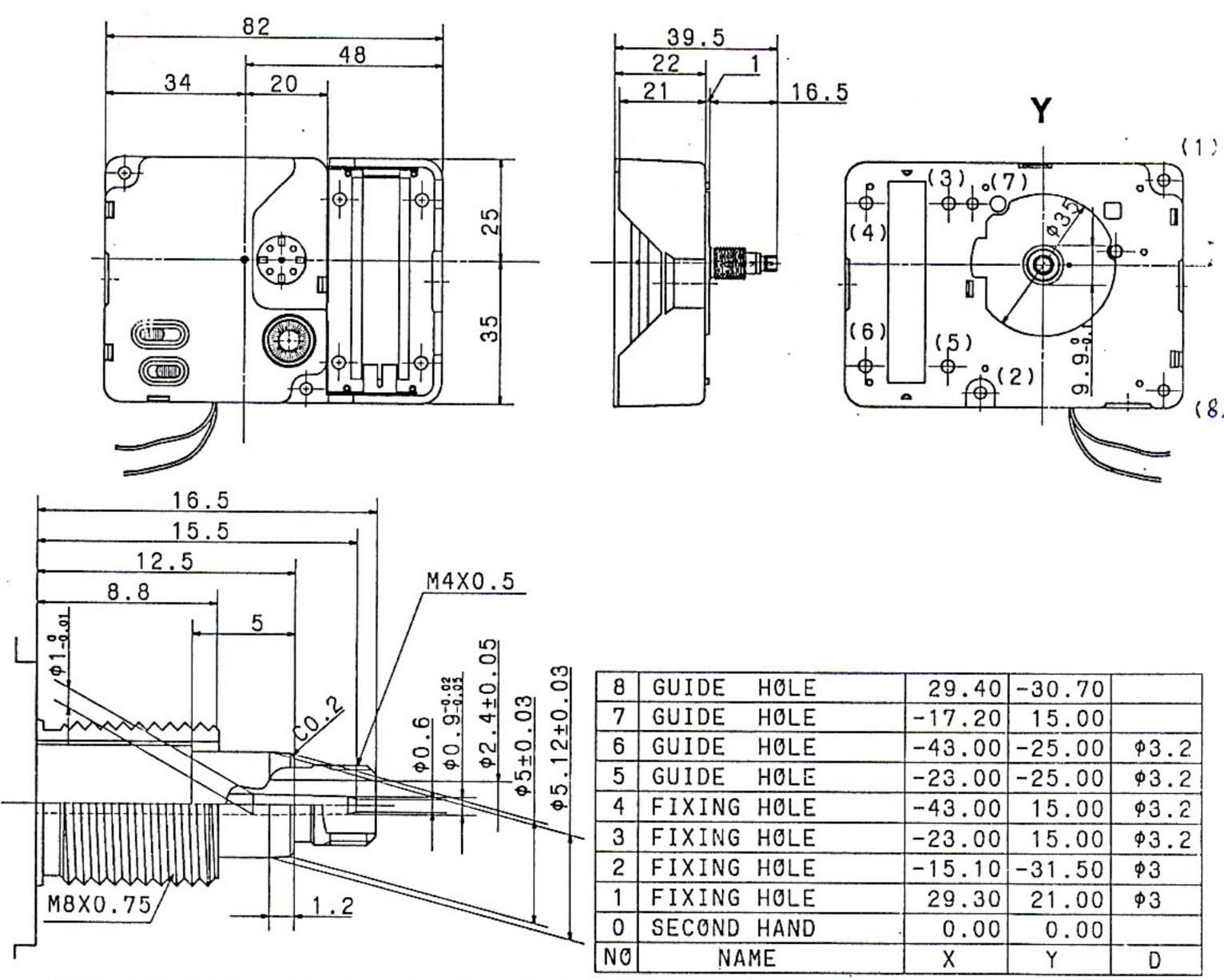
"Remark: There is a marking by cutiing the part of plastic hour hand shaft on the 12:00 position."
